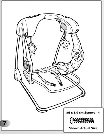
• Insert two #6 x 1.9 cm screws through the upper swing arm and into the lower swing arm. Tighten the screws.
